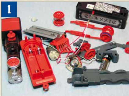
1 Removing the electric parts.
